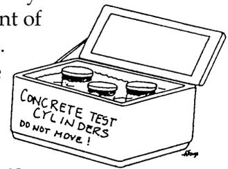
Cylinders should be carefully placed in the cooler and the cooler filled with water within 1 inch of the top of the cylinders.
