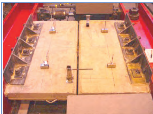
Figure A3-3 Lehigh Phase 1 test specimen and sample results for cyclic shear response (test & FE model) (right).
