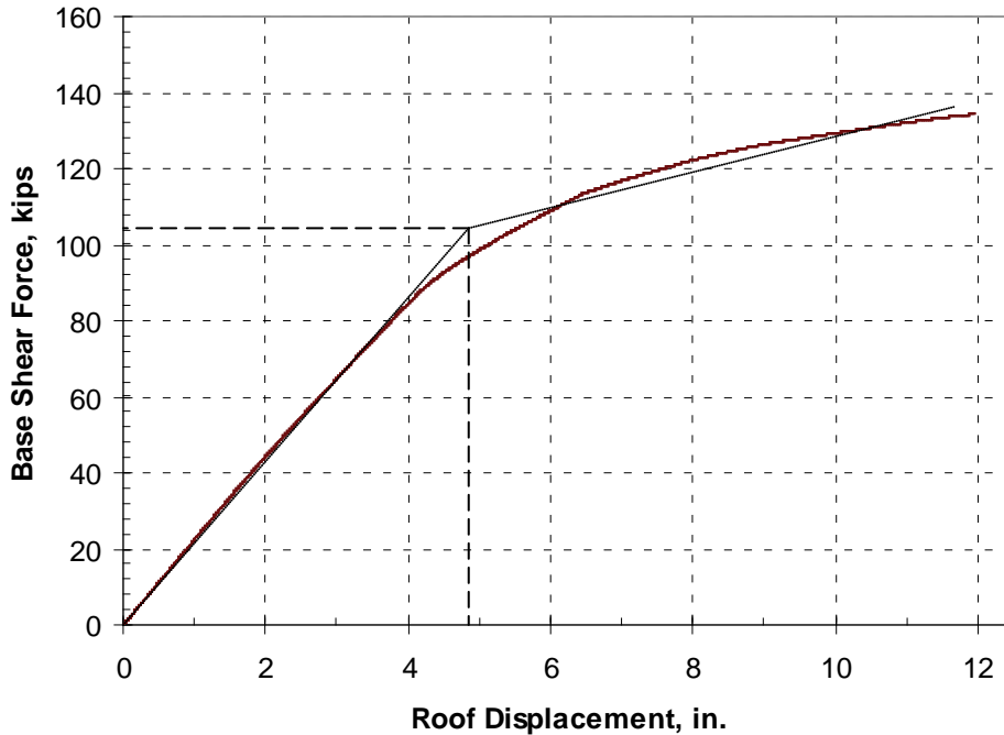
Figure 14 Capacity curve determined in a nonlinear static analysis of the reinforced concrete frame.
